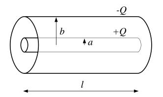
A cylindrical capacitor is constructed from two long concentric cylindrical conductors of length l and radius a and b (where a < b).
