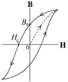
To measure - wind a coil around the specimen. H is determined by current in the coil. *B* is determined from integrating up the time-dependence of the voltage. [4]
