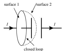
Line integral around loop must be independent of the surface bounded by the loop. But for surface 1 there is a current *I* penetrating it, but there is no current penetrating surface 2. So there is an inconsistency. [5]
