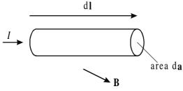
The force on the element of wire due to the applied magnetic field **B** is, from Equation (6.4)
