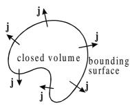
consider a closed volume, then the rate of decrease of charge in the volume must be balanced by the rate of flow of charge across the bounding surface. This may be expressed mathematically by
