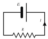
Kirchhoff's voltage law states that the sum of voltage drops and EMFs around a closed loop is zero. In this circuit this means that
